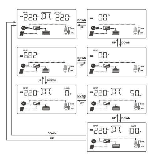
3.3.4.2 Main menu: in the main interface, long press function key for 5 seconds or less to enter the main menu, and press DOWN or UP to view the sub-menu. The function of P0/P1/P2/P3/P4 in the flashing state is as follows:
